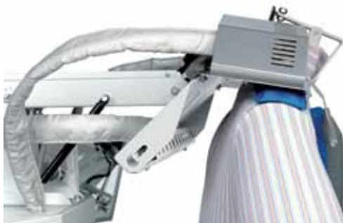
The press dries the upper seam without shine, because it is coated. A powerful jet of hot air dries the seam of the yoke without pressing it, therefore it does not leave a shine and does not ruin any darts and decorations. The width of the shoulders can be adjusted according to the cut for a wrinkle-free shoulder area, and can be corrected at any time during the cycle.
