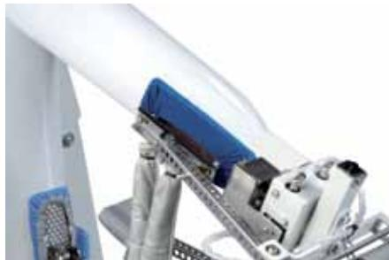
The rigid insert inside the sleeve ensures that the sleeve guards are perfectly ironed
