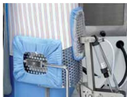
The tensioning carriage has five clamps to guarantee an even pressing of the hem, without crimping or horizontal lines. The number and intensity of the vertical tensioning movements performed by the carriage during the cycle can be programmed. When pressing delicate shirts, the tensioning clamps can be completely excluded by simply pressing one button on the console.
